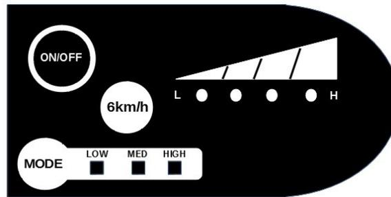
You can switch on the power supply of the e-bike motor by pressing the red button **ON/OFF** (*top, left*) for a few seconds. You can switch off the power supply of the e-bike motor by briefly pressing the red button **ON/OFF** (*top, left*).
