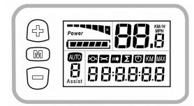
You can **switch on** the power supply of the e-bike motor by briefly pressing the **M** button (*left, middle*).
