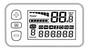
You can **switch on** the power supply of the e-bike motor by briefly pressing the **M** button (*left, middle*).
