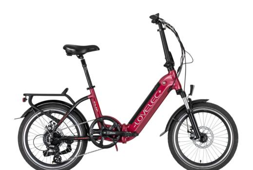
LG, Li-ion, 12,8 Ah (460,8 Wh), integrated battery:
